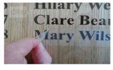
Take one corner of application tape and slowly remove in a downward motion at an angle as above image.
